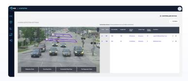
A dilemma zone at intersections is where a vehicle is too far to safely proceed through the intersection before the light turns red but too close to stop comfortably without sudden, potentially dangerous deceleration. This can cause rear end crashes and red light running.
