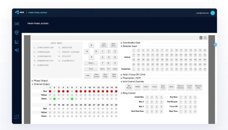
NoTraffic's Al Mobility Platform enables remote access to the front panel of a Traffic Signal Controller (TSC), addressing the challenges associated with unconnected cabinets and eliminating the need for signal technicians to travel to the site to operate the TSC.
